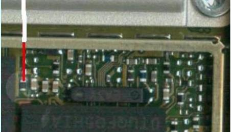
Here is a clear picture of where your wire Should connect to. This cable needs to GND it.
